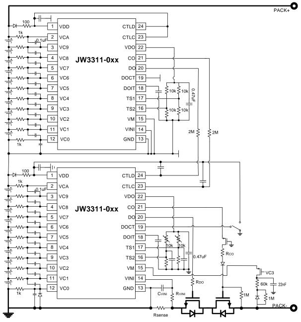
**Remark:** when the cell11~cell20 had over-discharge fault, the load lock function is disabled. If need the load lock function, please refer to "User Manual"
