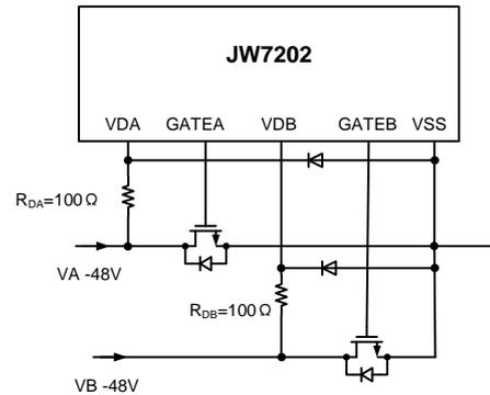
Figure 1. Method of Protecting the DA and DB Pins from Negative Inputs
