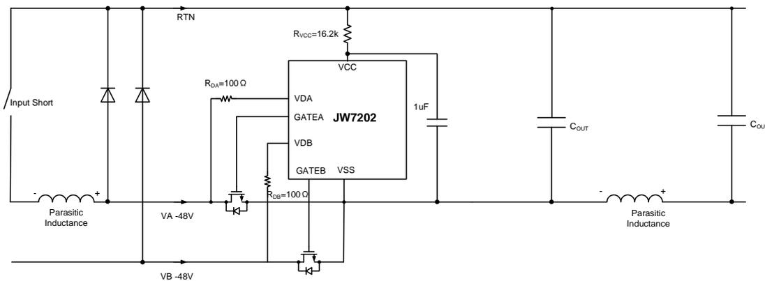
**Figure 2 Input Supply Fault Transients**
