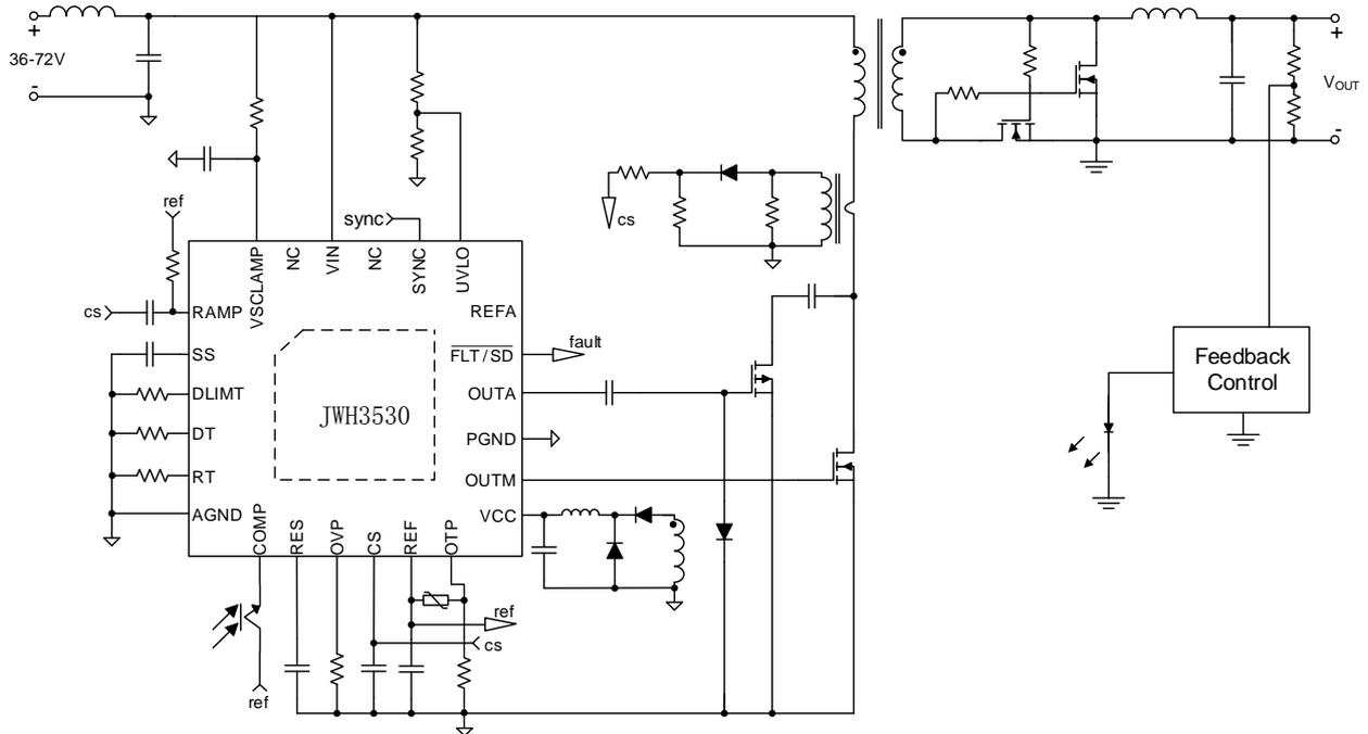
Figure 2. Typical application circuit with current mode control
