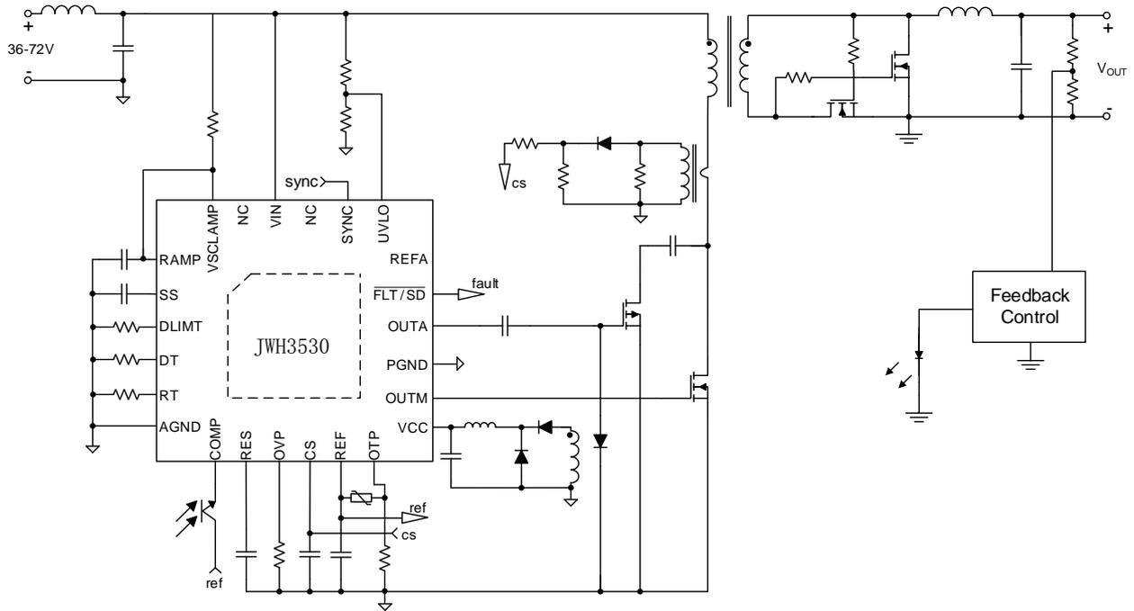
Figure 1. Typical application circuit with voltage mode control
