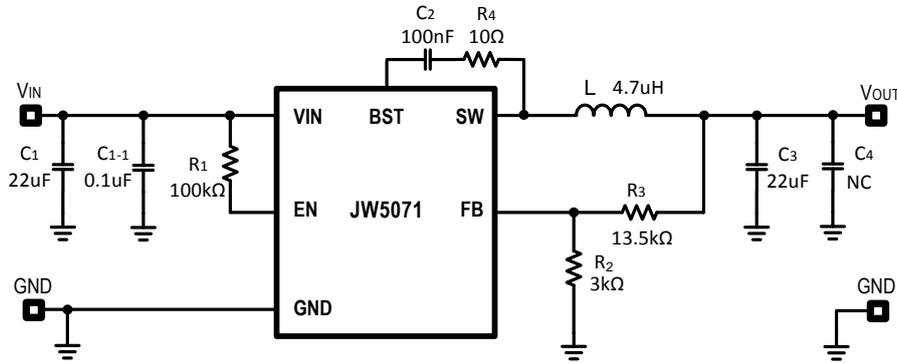
Figure 6:  $V_{IN}=24V$ ,  $V_{OUT}=3.3V/2A$
