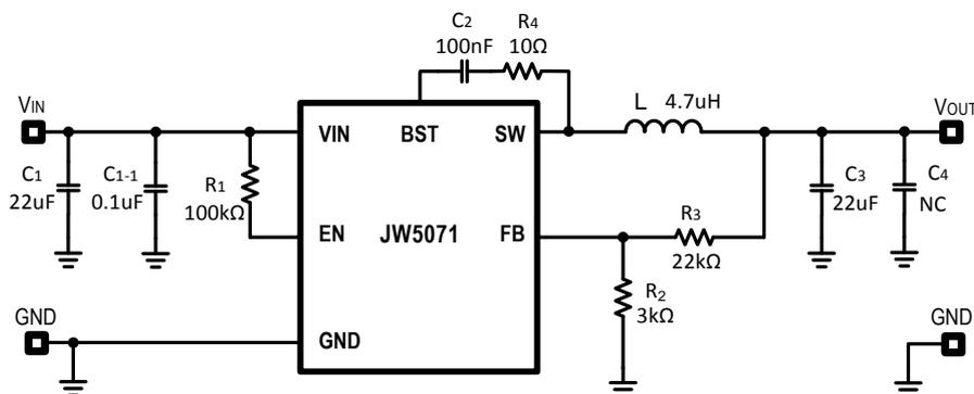
Figure 8:  $V_{IN}=24V$ ,  $V_{OUT}=5V/2A$
