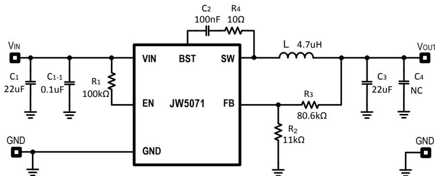
Figure 7:  $V_{IN}=12V$ ,  $V_{OUT}=5V/2A$
