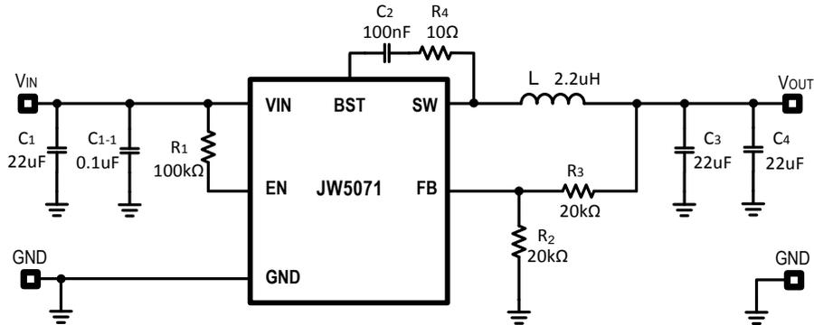
Figure 3:  $V_{IN}=5V$ ,  $V_{OUT}=1.2V/2A$
