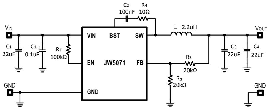
Figure 4:  $V_{IN}=12V$ ,  $V_{OUT}=1.2V/2A$
