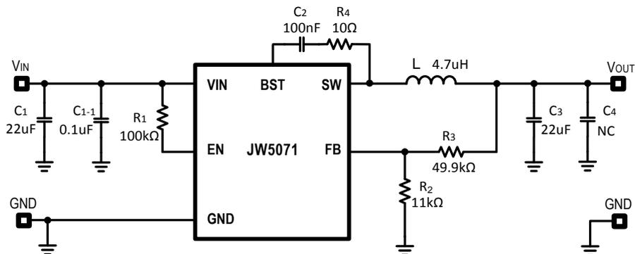
Figure 5:  $V_{IN}=12V$ ,  $V_{OUT}=3.3V/2A$
